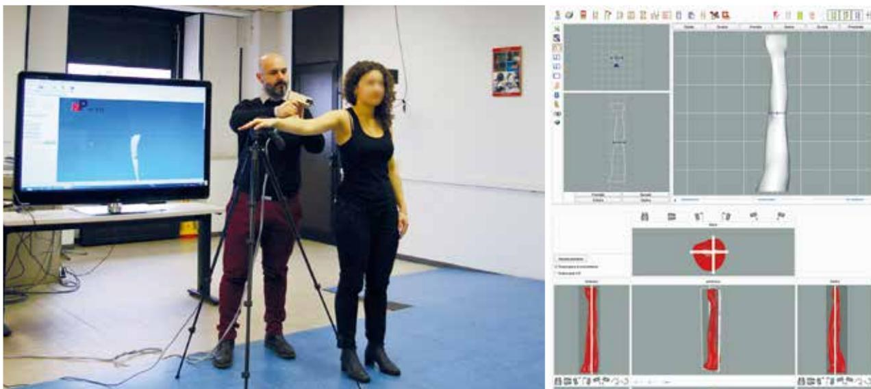
From left to right: the portable 3D scanner being used in the study; 3D acquisition of a limb with lymphedema by laser scan; Data processing with the analysis software
